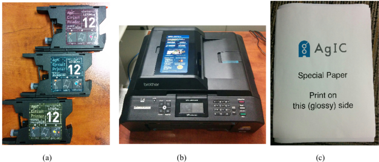
Figure 1. Spoof creation. (a) Three AgIC silver conductive ink cartridges, (b) Brother MFC-J5910DW printer, and (c) AgIC special paper.
