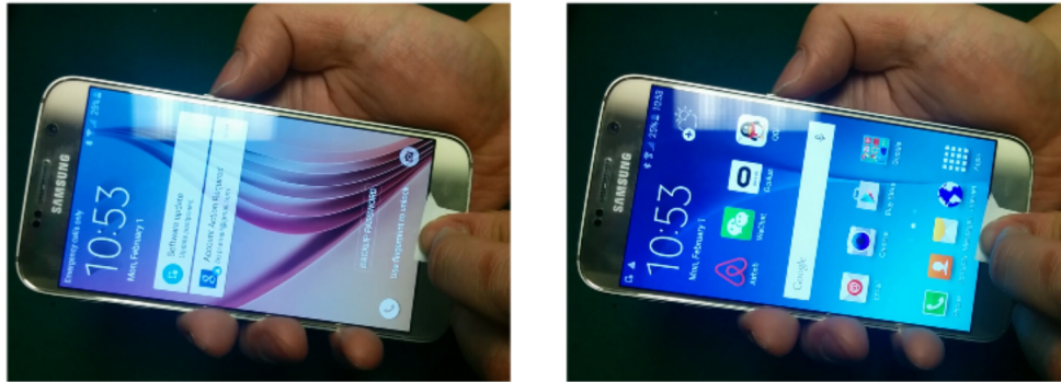
Figure 3. Unlocking Samsung Galaxy S6 using a printed 2D fingerprint image in Figure 2 (b).
